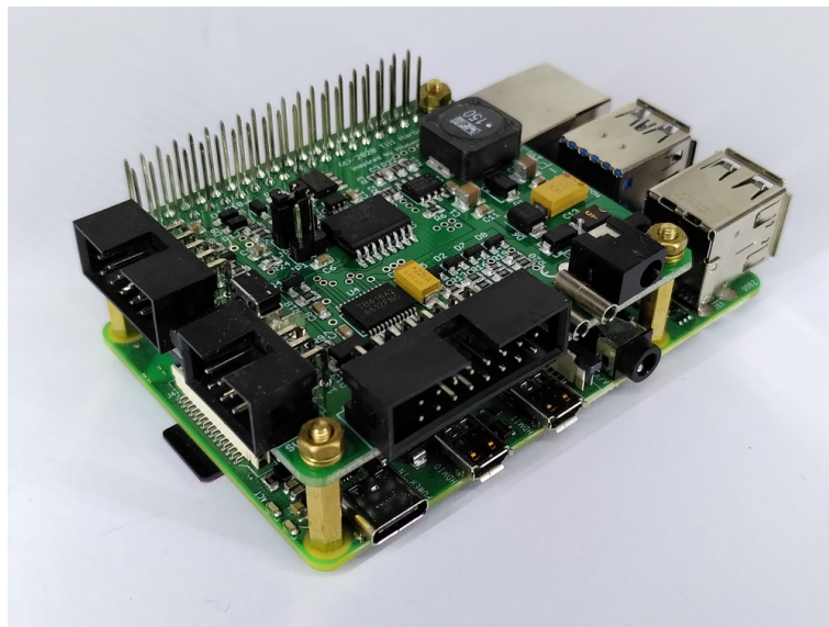
Figure 2.1: The ft HAT mounted on a Raspberry Pi
